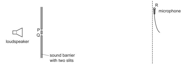
What is the condition for an intensity maximum (loud sound) to be detected by a microphone at R?
