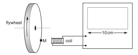
The flywheel has a small magnet M mounted on it. Each time the magnet passes the coil, a voltage pulse is generated, which is passed to the c.r.o. The display of the c.r.o. is 10 cm wide. The flywheel is rotating at 3000 revolutions per minute.
